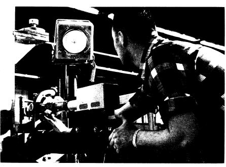
TV OPTICAL TOOLING—A closed circuit television system that can cut costs and speed production of supersonic fighter-bombers has been developed by Republic Aviation Corporation. Previously a two-man operation in an optical tooling process, now the TV camera automatically "looks" through the telescope while the operator positions jig contour plates by lining up cross-hair patterns as they appear on the TV screen.
