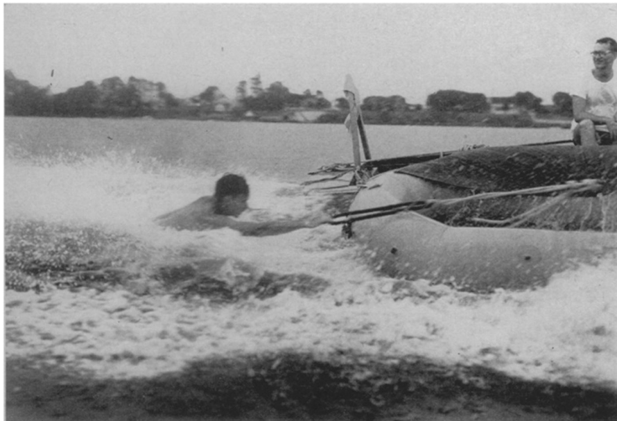
RESCUE DEVICE —The frogman being rescued in this picture is actually traveling faster than the rescue boat. He is being drawn in by the tensioned cord which works like the released rubber band in a slingshot.
