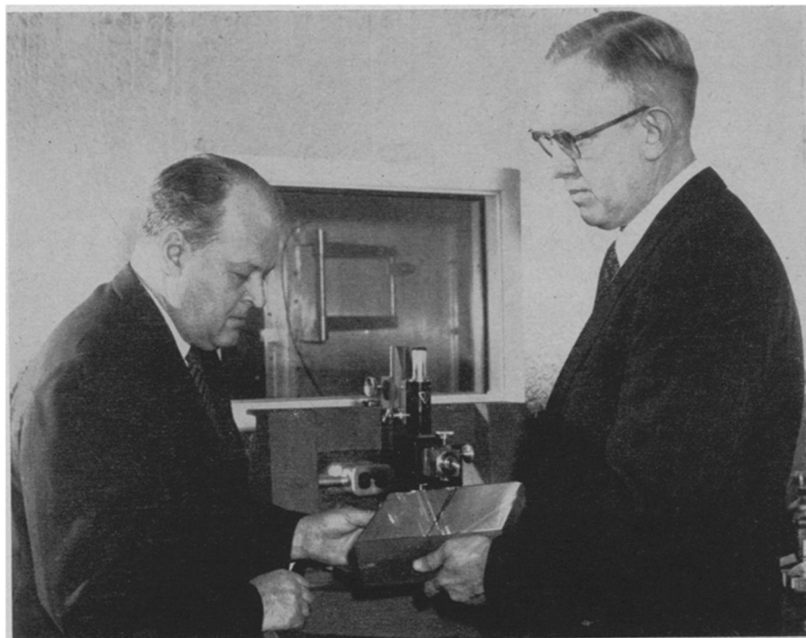
ANTARCTIC INSTRUMENT —This looks like an ordinary block of glass, but actually the surface has been cut with minute lines, 15,000 to the inch and each line is exactly 20 millionths of an inch deep. The diffraction grating, produced by Bausch and Lomb Optical Co., will play a key role in France's participation in the International Geophysical Year. It is being examined by S. W. Steensma and David Richardson of B & L.
