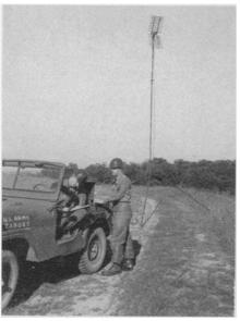
RADAR RULER — Two separate jeep-portable radar stations, one at each end of the distance to be measured, constitute the system developed by the Army's Signal Corps Engineering Laboratories at Fort Monmouth, N. J., for surveying great distances when long-range and speed are essential. Using it, 50 miles can be measured to within a few feet.
