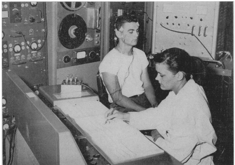
TESTING FOR JETS —This combination instrument records brain waves and provides a fast and accurate analysis. It helps to measure certain physiological changes affecting the shape and frequency of brain waves.
