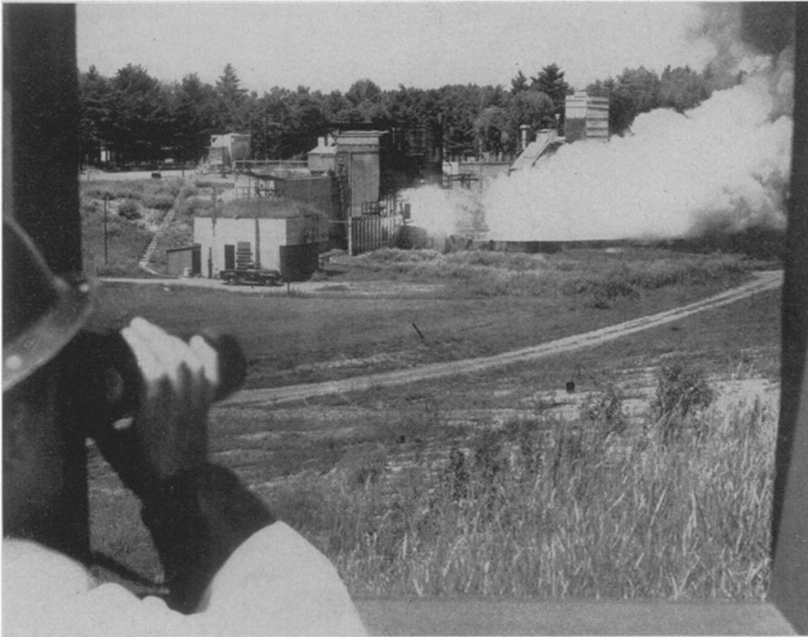
SATELLITE ROCKET TEST —The rocket engine that will furnish the initial push for launching the earth satellite during the International Geophysical Year is watched from a bunker house as it goes through trial runs at Schenectady, N. Y. The General Electric X405 burns a hydrocarbon fuel and liquid oxygen.
