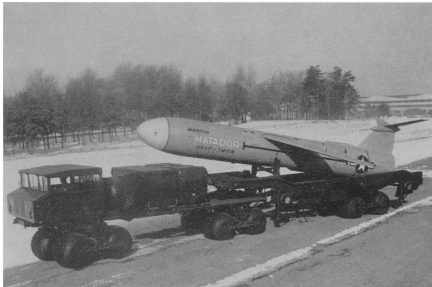
MARTIN MATADOR —The TM-61B Martin Matador, a new surface to surface guided missile, made its appearance in the President's inaugural parade. It is shown with its launcher and towing vehicle. The latter two vehicles are both of revolutionary design and are capable of carrying the missile and all support and launching equipment to previously inaccessible launching sites.
