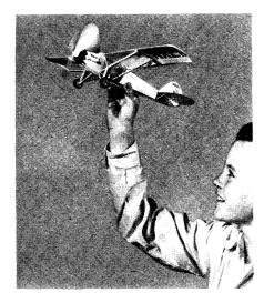
plane is 11 and one-half inches long and has a wing span of 18 inches, as shown in the photograph. It is powered by a rubber hand.
