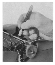
cluding crude, and is designed to pick up all excess oil after application. Useful for oiling typewriters, as shown in the photograph, cameras, guns, lathes, precision machinery and electronic devices, the instrument functions at any angle, even upside
