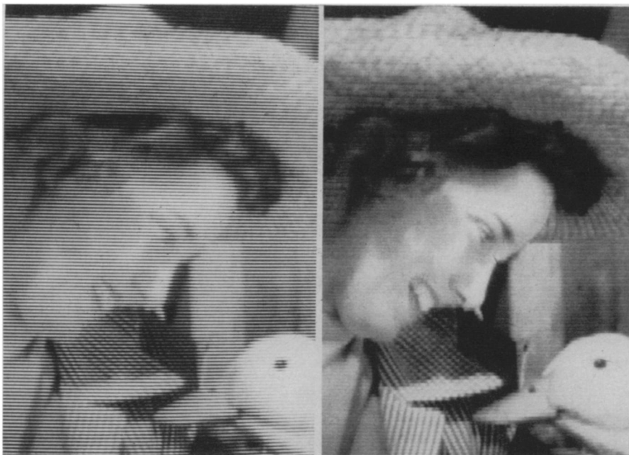
"WOBBLING" —A method of line structure reduction in which the electron beam is "wobbled" gave the improved television picture shown at the right in these actual photographs of the same tube. The left picture is "normal."
