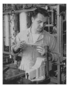
PIPEFUL OF PLATINUM - Platinum catalyst is being loaded into a pipe for use in Gulf Oil Corporation's newly developed bydroisomerization process. Behind operator Eugene M. Gatty stands one of the experimental units at Gulf's Harmarville, Pa., research center. The bulk supply of high octane fuel could be increased by possibly 20% as a result of this process.
