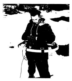
the operator by shoulder harnesses. One wears a receiving coil, and the other a transmitting coil. The two pieces of equipment are connected by a 200-foot cable.
