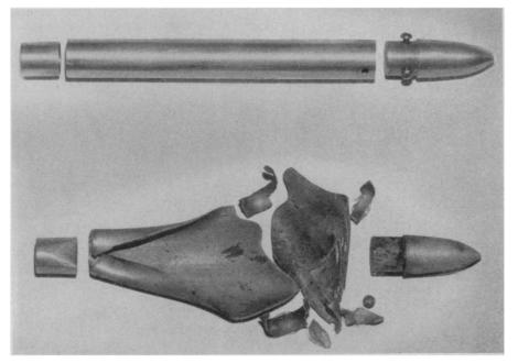
WRONG FUEL SPELLS DISASTER—A well-constructed amateur rocket, such as the seven-inch, heavy-gauge aluminum student rocket shown at the top, can be a safe, instructive scientific instrument when handled properly. Lt. Col. Charles M. Parkin Jr., who warns against blasting caps and black powder as dangerous fuels, "launched" an identical model inside a container. Fragments at the bottom resulted from loading with a small charge of black powder.
