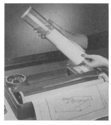
outlet and can be adapted for use in automobiles, boats or planes. Copy and paper are placed in a butyrate plastic tube and exposed to a fluorescent lamp.
