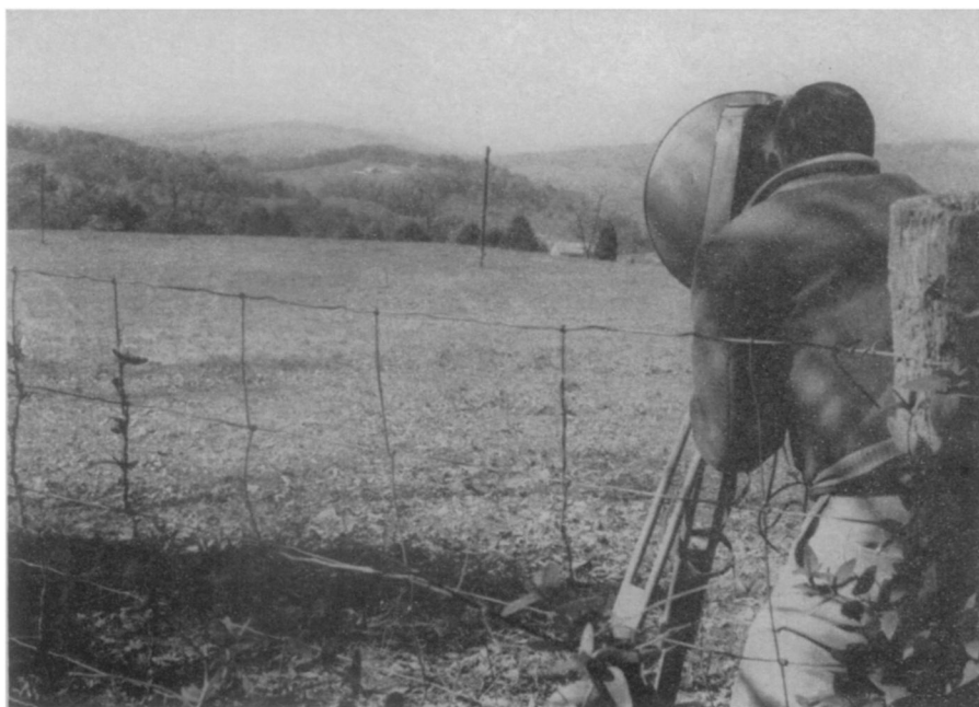
ELECTRONIC SURVEYING —Engineers using an electronic technique developed by Tellurometer, Inc., Washington, D. C., can be miles apart and out of sight of each other and yet measure distances with a maximum error of 11 inches in 40 miles. A surveyor, shown in the photograph, operates a small radar transmitter sending microwaves to a distant receiver. The time it takes the waves to make the round trip gives the distance.
