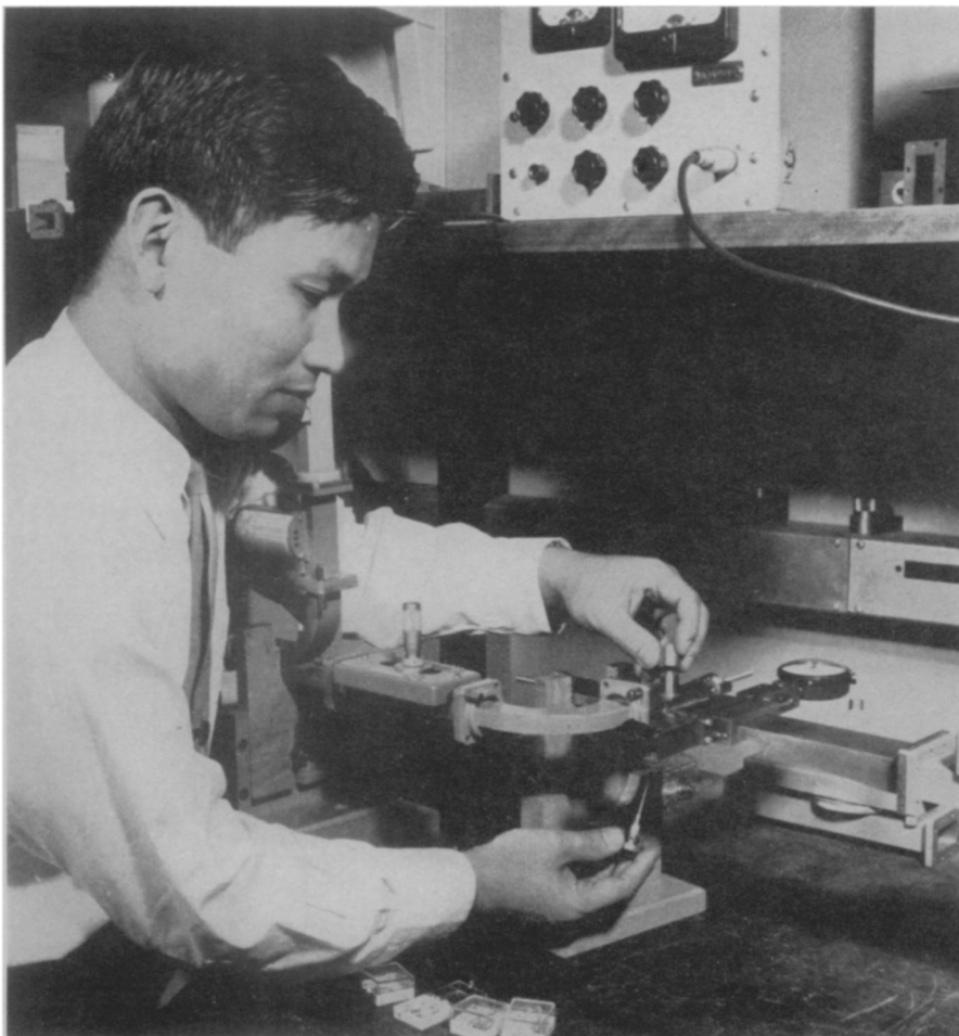
LOW-NOISE AMPLIFIER —A new low-noise ultra-high frequency and microwave amplifier now under development at Bell Telephone Laboratories uses special semiconductor diodes. M. Uenohara mounts a diode in a waveguide structure for checking its amplifying properties.
