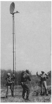
READY RELAY—The 20-foot mast and two-and-one-half-foot reflector used by the Marine Corps radio relay set goes up in minutes in the field. Using an extremely narrow message band, the radio operates in super high frequency range and can "send" for a distance of 40 miles. The Raytheon Manufacturing Company, Waltham, Mass., will supply the radio relay sets.
