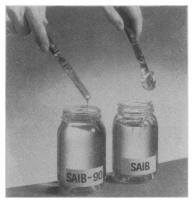
SAIB has a viscosity of 100,000 cps at 86°F. Add 10% ethyl alcohol, making SAIB-90, and the viscosity drops to 700 cps. Any of the commercial lacquer solvents thins it similarly.
