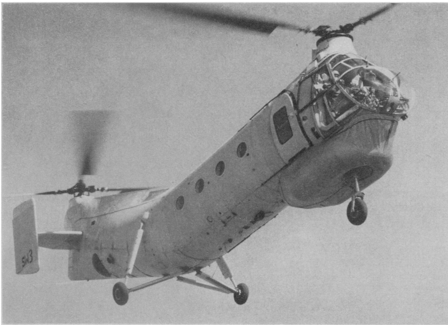
HANDS-OFF HELICOPTER —A helicopter is precisely stabilized during a "hands-off" flight (note pilot) as a result of an automatic flight control system developed by the Sperry Gyroscope Company, Great Neck, N. Y. Complete four-axis control, pitch, roll, heading and altitude, is provided in the system which takes its commands directly from the pilot's controls. Electronic trimming, automatic turn coordination and push-button controls for precise attitude adjustment are among the system's automatic features.
