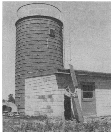
TEST TOWER —The rain-erosion test tower, recently erected at the B. F. Goodrich Company Research Center, Brecksville, Ohio, is shown here along with the rotor blade.
