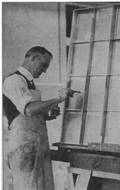
RETOUCHING one of the wide metal culture trays with acid-proof lacquer
