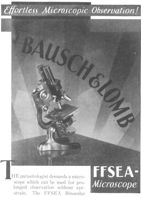
Microscope not only relieves eyestrain but the interpupillary and eyepiece tube adjustments enable the user to set it to meet his optical requirements.
