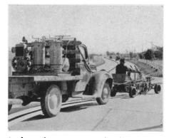
tanks and a compressor for feeding the markers. The latter consist of atomizing spray guns provided with side shields which assure clean-cut lines.
