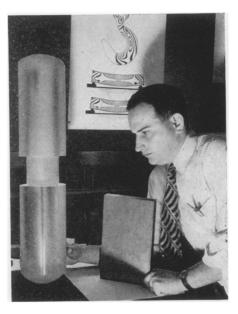
STRESSES AND STRAINS—These are revealed by use of plastic counterparts in operating machinery which can be examined under polarized light.
