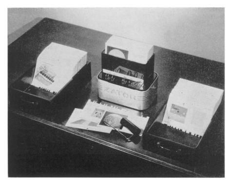
CHEMICAL ZATOCODING—Simple codes are used for complicated chemical names for indexing purposes which, by means of mechanical sorting according to the random pattern notches, afford an easy method of picking out any desired combinations of chemical or other properties.
