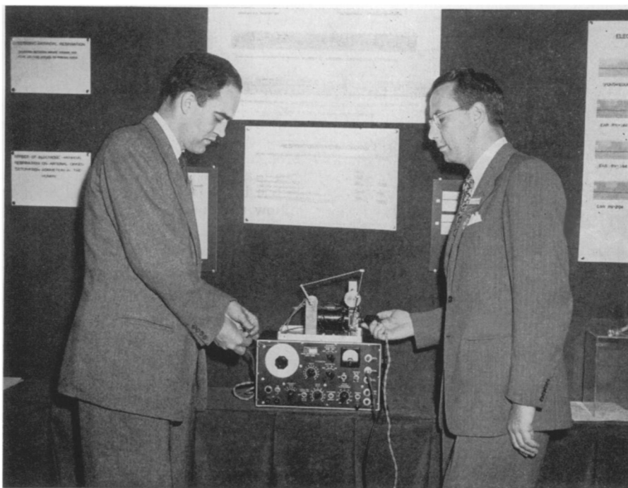
ELECTRONIC RESPIRATOR —This experimental model, which may prove to be an iron lung substitute, is demonstrated by Drs. James W. Whittenberger and Stanley J. Sarnoff of Harvard. When produced for general use, it will be only about half this size and have fewer dials and knobs. Dr. Whittenberger at left is holding the silver electrode that is attached to the patient's phrenic nerve through a small cut in the neck.
