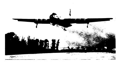
SIX-JET BOMBER—Undergoing military tests at Wright Field, Ohio, by the U. S. Air Force, is the largest jet bomber of conventional design yet put in the air. It was built by Glenn L. Martin near Baltimore, Md., and for the present will be known as the XB-48. The X will be dropped when tests are completed and the bomber accepted. It will then go into production.
