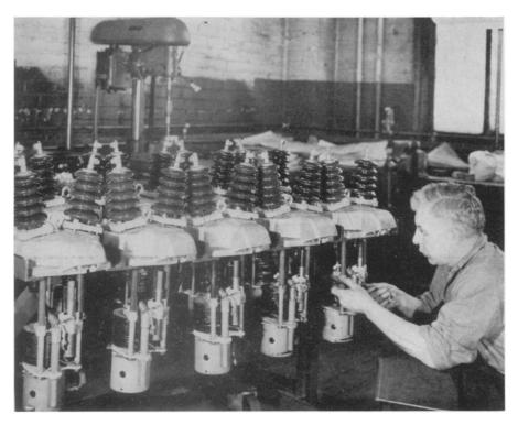
GUARDIANS OF RURAL ELECTRIC SERVICE—These devices, called GR circuit reclosers, will be installed on rural electric lines to guard against prolonged service interruptions. These units reclose the electric circuits automatically following such interruptions as might be caused by overloads, short circuits or other temporary difficulties. The work is being done at Westinghouse Electric Corporation's East Pittsburgh Works.
