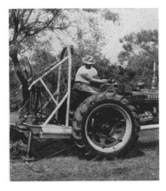
TREE-PULLER, shown in the picture, is used in connection with a farm tractor and lifts reasonably large trees out of the ground, roots and all. Two powerful jacks, which rest on the ground at the rear, and a pair of gripping jaws are used, the jacks being powered by the tractor engine.
