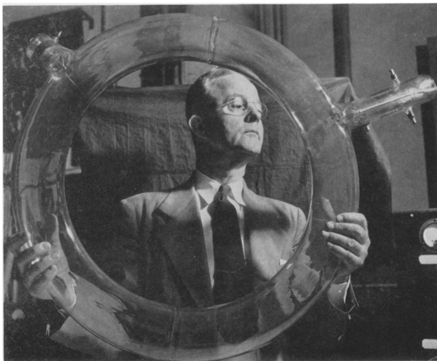
50,000,000-VOLT X-RAYS —Heart of a recently completed betatron in the General Electric Research Laboratory, is this glass "doughnut" being examined by Dr. Ernest E. Charlton, head of the X-Ray section. Electrons, emitted from a hot filament inside this vacuum tube, are whirled around thousands of times. As acceleration builds up the magnetic field to its maximum, the orbit of the whirling electrons is shifted and they hit a tungsten target which they missed before. This generates a beam of high-voltage X-rays, and occurs at the rate of 60 times per second.
