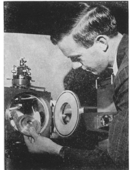
ELECTRONS AID IN METAL STUDY —Dr. J. G. Hutton is shown inserting a sample into the electron diffraction instrument which is used to study corrosion and crystal structure of metal in General Electric Company's laboratory.
