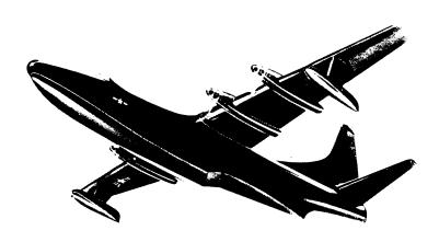
PATROL FLYING BOAT—This is an artist's conception of the XP5Y-1, two of which are being built for the U. S. Navy by Consolidated Vultee Aircraft Corp. of San Diego. It has a quick take-off and high speed due to its four powerful, propeller turbine, Allison engines and is designed for long-range day and night search of sea areas, rescue operations, and anti-submarine patrol. The first experimental XP5Y-1 is expected to fly early in 1949.
