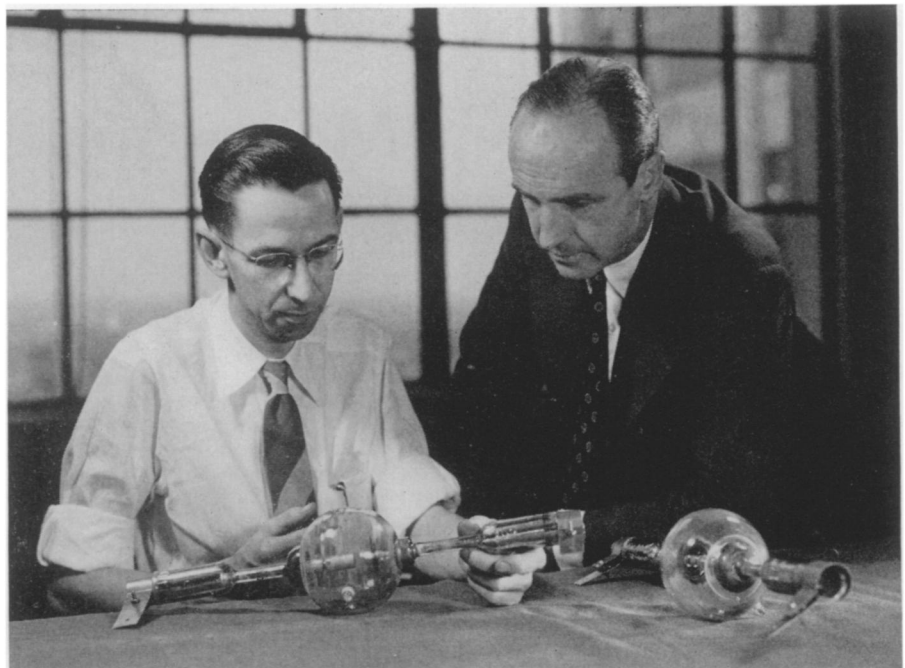
HIGH POWER LIGHT —The experimental 10,000-watt movie lamp which is for direct current operation is shown at the left and a similar lamp for alternating current circuits is at right.
