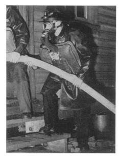
SELF-BREATHING APPARATUS for firemen, shown in the picture, is for use in smoky fires and gas-filled rooms where oxygen is not otherwise available. The breathing bag, which fits over the chest, contains a canister of potassium tetraoxide
