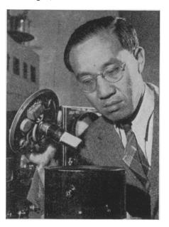
TINY ATOM-SMASHING MA-CHINE—This Westinghouse device is in reality a neutron counter which detects neutrons, vital building blocks in matter's structure which carry no electric charge. It is demonstrated by Dr. Kuan-Han Sun, Chinese-born Westinghouse research physicist. Containing a very small amount of uranium 235, it generates tiny atomic explosions to reveal the neutrons.
