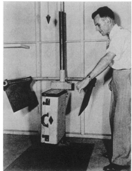
FOR MORE DURABLE LUGGAGE —A luggage smashing machine is shown in operation to determine the resistance to strain of the baggage. Tests closely duplicate stress encountered in travel.
