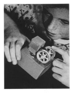
TINY POWER UNIT for toys, shown in the picture, is operated by two standard flashlight batteries which are inserted at will in the plastic base-box of the engine, and delivers power by moving belt
