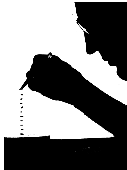
ULTRASONIC STUNT — Bits of cork are suspended ladder-fashion in mid-air by ultrasonic waves. The sound is coming from an air whistle, smaller than a cigarette, located two feet above the tweezers.
