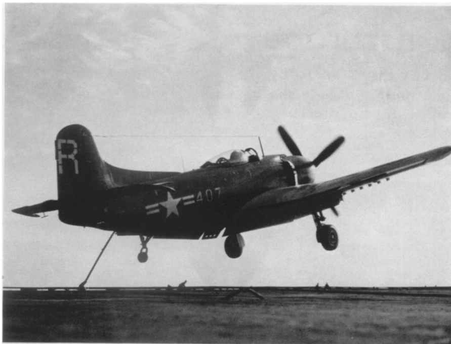
OVER-SIZE CARRIER-BASED PLANE —The Navy's newest attack plane, a Martin AM-1 Mauler, is shown making contact with the cable which will bring this largest and most powerful plane ever to operate from a flattop's deck to a swift, safe halt.
