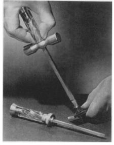
so that the shaft can be spun without raising a blister on the palm of the hand. The movable hammer head, which can be fixed anywhere along the shaft by a set-screw, may also be used as a fist-grip for stubborn screws.
