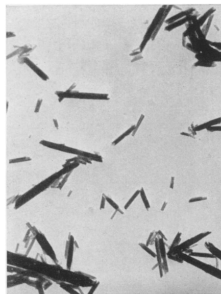
TINY TUBES FORM CLAY —This tubular structure of a common red clay called halloysite was discovered by studies with an electron microscope, which magnified the clay up to 60,000 times. This picture of halloysite and other clays was made at Pennsylvania State College by Thomas F. Bates, Fred A. Hildebrand and Ada Swineford.
