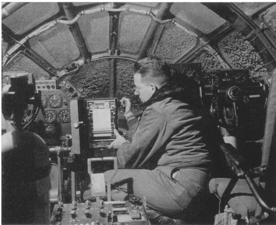
FLIGHT RECORDER —The device automatically records air roughness, altitude, and operation of automatic pilot and de-icing equipment on aircraft. It is being checked here in a B-29 Flying Laboratory at General Electric Flight Test Center near Schenectady, N. Y.
