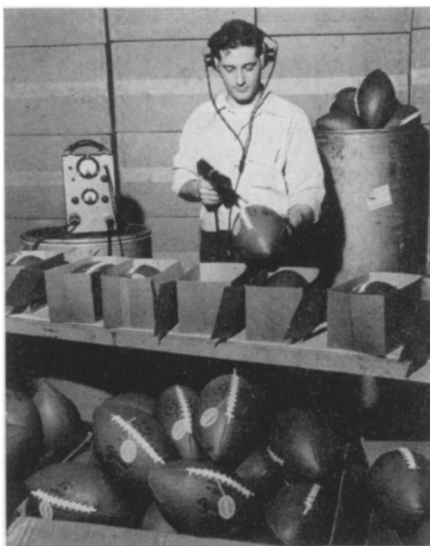
if the air contains gases of the Freon group. Footballs under test are filled with such a gas.
