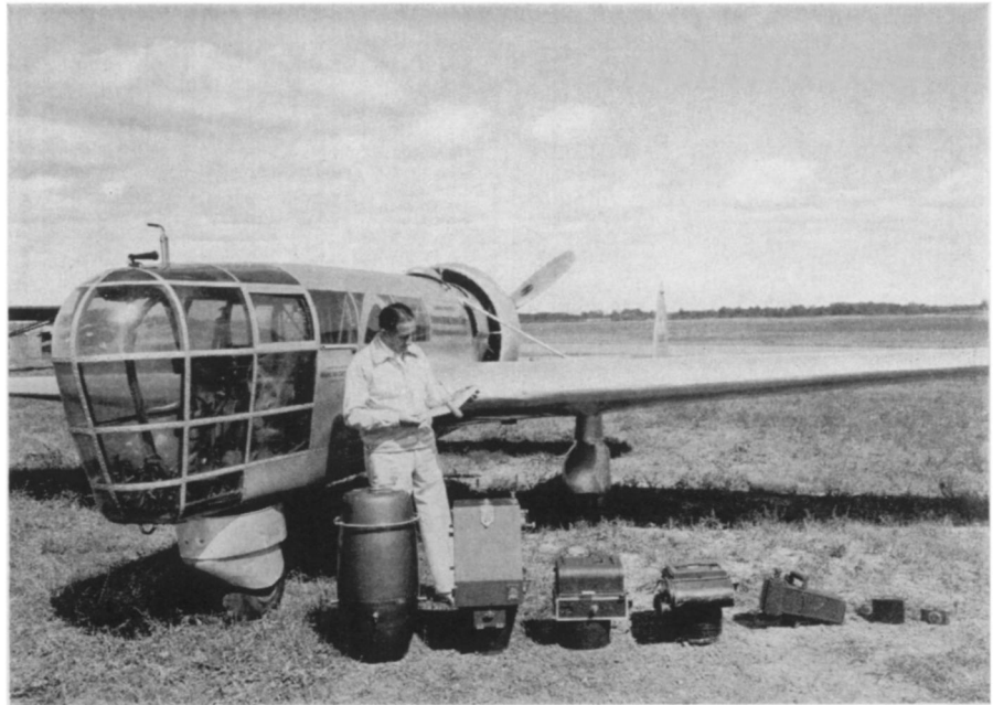
PHOTOGRAPHIC SHIP —Beside the "Explorer" is shown its builder, Talbert Abrams, who examines a model of a proposed new "Explorer II". Shown also are various aerial cameras used aboard the photographic plane.
