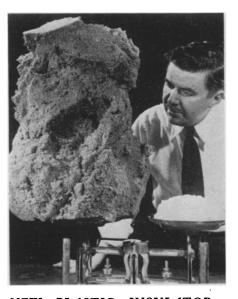
NEW PLASTIC INSULATOR— The plastic foam balances pie meringue on these scales because, despite the great difference in volume, they both weigh the same amount —five ounces. Making the weight comparison is Robert Sterling, Westinghouse chemist who developed the insulating material. bles of air as the solidified plastic is exposed to the air. The solid plastic piece contains only one part of resin to 100 parts
