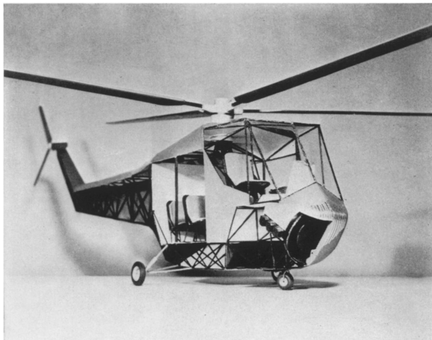
AGRICULTURAL CRAFT —Dubbed the Pelican, this model shows the cab-over-engine arrangement of a new helicopter which permits location of payload astride the ship's center of gravity. It can also be converted to carry six passengers in addition to the pilot.
