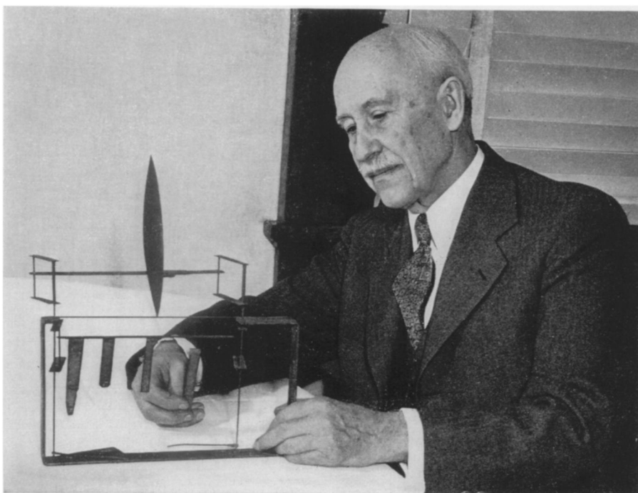
WRIGHT WIND TUNNEL INSTRUMENT —Here the late Orville Wright is shown with one of the simple but effective wind tunnel instruments devised by the Wright Brothers. Their original instruments have been bequeathed to the Franklin Institute in Philadelphia.
