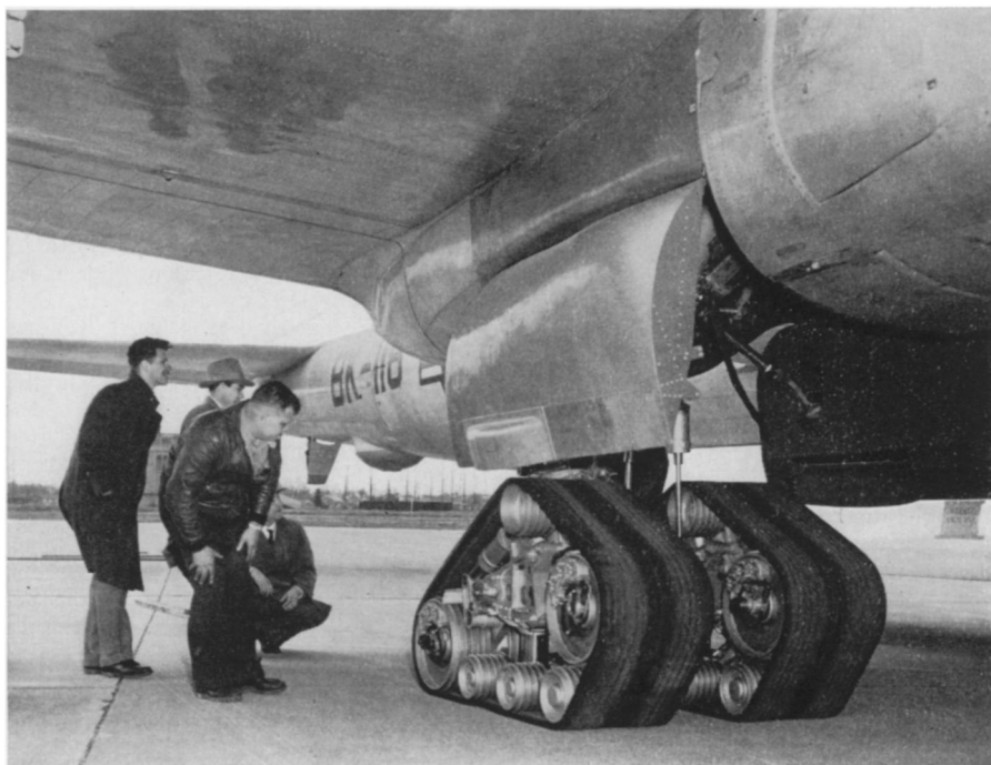
TRACK-TREAD LANDING GEAR —Mounted on a Boeing B-50 Superfortress, this installation is the largest of its type ever built and will be used in testing the practicality of flying heavy airplanes from unimproved airfields.
