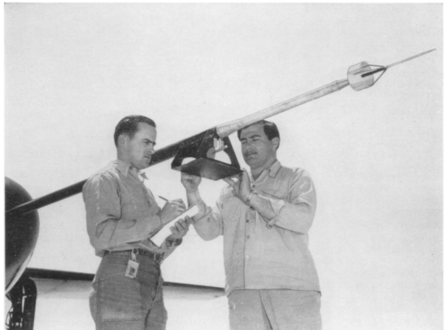
FLIGHT-CONDITIONS DETECTOR —Sensory devices are housed in this long, needle-like boom which is supported well ahead of the nose of a Northrop Scorpion XF-89 all-weather fighter. Detectors transmit electronically to recording instruments in the plane such information as air speed, altitude, and yawing action.
