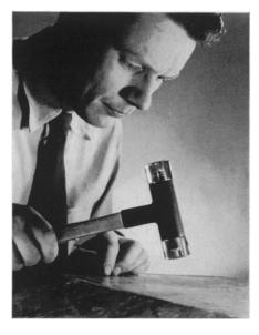
relatively soft plastic faces, and a hollow metal head between them, which contains a charge of steel grit. As the tip is lowered, the charge follows, practically eliminating recoil of the hammer after it has struck. The plastic tips withstand heavy impact without cracking or flaking.
